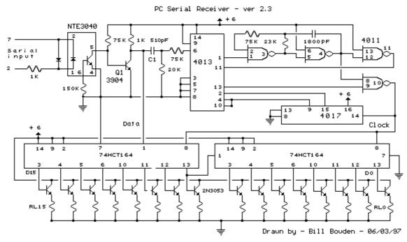
This circuit was designed to control a 32 channel Christmas light show from the PC serial port. Originally designed with TTL logic, it has been simplified using CMOS circuits to reduce component count. It is a fairly simple, reliable circuit that requires only 4 common CMOS chips (for 8 outputs), an optical isolator, and a few discrete components. The schematic diagram (SERIAL.GIF) illustrates the circuit with 16 outputs which can be expanded with additional 8 bit shift registers.
